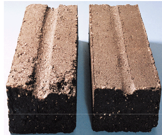
Beam specimen after rutting test
